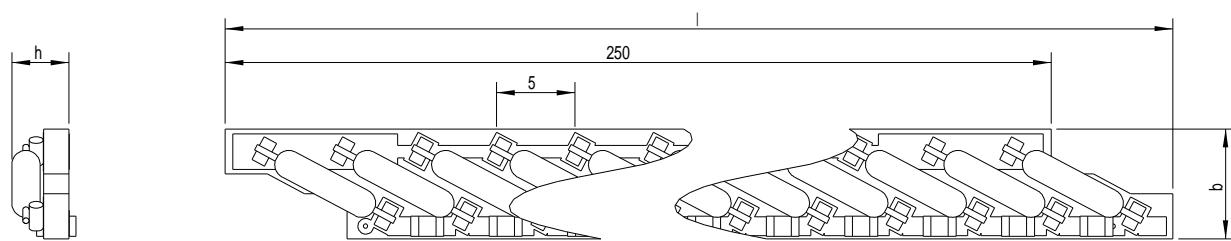
(All switches are arranged in an angle of 28° and in a pitch of 5mm. The blades are oriented randomly.)
